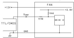
$V_{\text{CONT}}$  is above 2.0 V  $\cdots$  Fan should run full speed.
