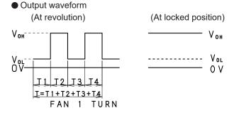
Remark: At locked position, output becomes  $V_{OH}$  OR  $V_{OL}$   $T=T_1+T_2+T_3+T_4=60/N$  (Sec)
